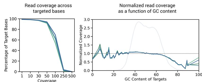
**Figure 4.** Coverage and GC bias metrics. (A) Read coverage across targeted bases. Coverage values are derived from Picard tools CollectHSMetrics. (B) Coverage uniformity as a function of GC content. Values represent the relative read coverage over panel target regions of a given GC content, normalized to the mean coverage across all target regions. Gray line indicates frequency of targets by GC content.
